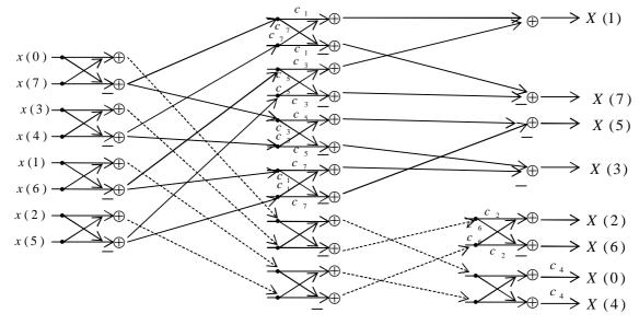
Figure 1: 8-point Discrete Cosine Transform
