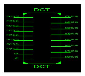
Figure 4: Resister transfer Level (RTL) View of 8-point DCT
